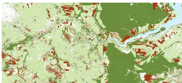
How it works: the European Space Agency's Sentinel-1 satellites scan the ground; with AI, all pixels that underwent change are detected. Vegetation clearing including deforestation is shown in red; intact forests are shown in dark green, and plantations are in light green. Source: Satelligence
